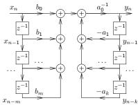
$$H(z) = \frac{b_0 + b_1 z^{-1} + b_2 z^{-2} + \dots + b_m z^{-m}}{a_0 + a_1 z^{-1} + a_2 z^{-2} + \dots + a_k z^{-k}}$$
