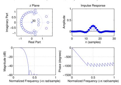
order: n=30, cutoff frequency (-6 dB):  $f_c=0.25 \times f_s/2$ , window: Hamming MATLAB DSP Toolbox functions: b = fir1(30, 0.25), zplane, impz, freqz, freqzplot
