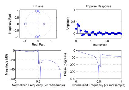
order: 5, cutoff frequency:  $0.5 \times f_s/2$ , pass-band ripple: -3 dB, stop-band ripple: -20 dB
