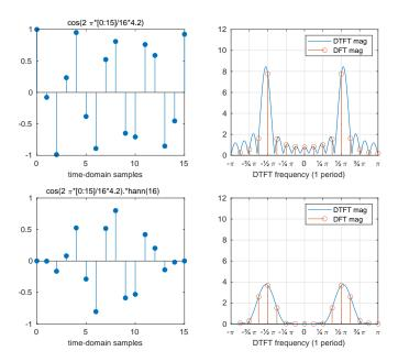
Numerous alternatives to the rectangular window have been proposed that reduce leakage and scalloping in spectral estimation. These are vectors multiplied element-wise with the input vector before applying the DFT to it. They all force the signal amplitude smoothly down to zero at the edge of the window, thereby avoiding the introduction of sharp jumps
