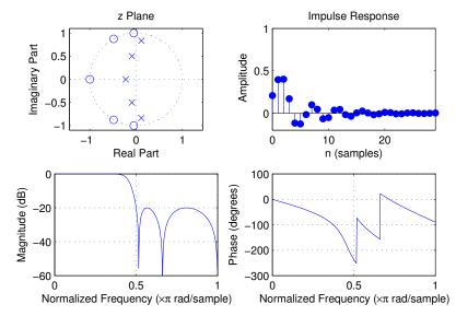
order: 5, cutoff frequency:  $0.5 \times f_s/2$ , stop-band ripple: -20 dB
