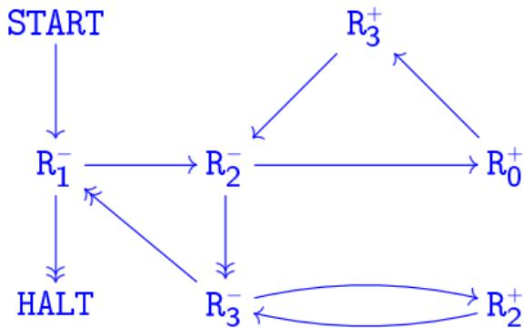
If the machine is started with  $(R_0, R_1, R_2, R_3) = (0, x, y, 0)$ , it halts with  $(R_0, R_1, R_2, R_3) = (xy, 0, y, 0)$ .
