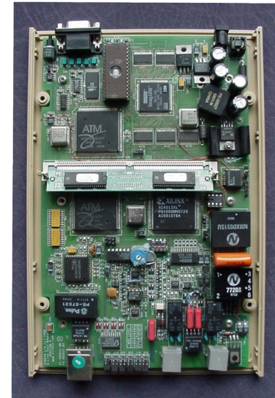
Prototype ADSL modem (DJG 1995)
