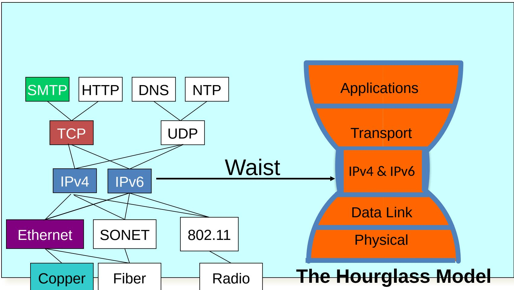
There is just <sup>TWO</sup> ~~one~~ network-layer protocol, IPv4 + v6
