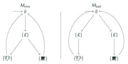
A G ( $\mathcal{E} \to E \times \mathbb{E}$ ): "For all paths, at every state (along the path) in which money has been paid, there exists a path from this state in which, in the next state, the machine has produced coffee."
