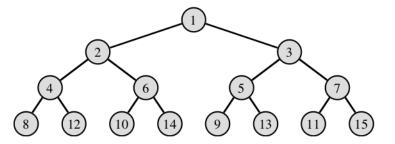
This simple representation (credited to W. Braun) ensures that the tree is balanced. Complexity of access is always  $O(\log n)$ , which is optimal. For actual running time, access to conventional arrays is much faster: it requires only a few hardware instructions. Array access is often taken to be O(1), which (as always) presumes that hardware limits are never exceeded.
