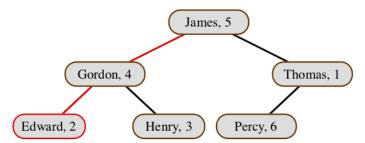
Binary search trees are an important application of binary trees. They work for keys that have a total ordering, such as strings. Each branch of the tree carries a (key, value) pair; its left subtree holds smaller keys; the right subtree holds greater keys. If the tree remains reasonably balanced, then update and lookup both take  $O(\log n)$  for a tree of size n. These times hold in the average case; given random data, the tree is likely to remain balanced.
