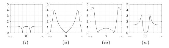
The z-transform of each impulse response has two zeros and two poles. Each zero or pole is at one of these 12 possible locations:  $e^{\pi j k/4}$  with  $k \in \{0, \ldots, 7\}$  or  $0.6 \pm 0.6 j$  or  $-0.5 \pm 0.5 j$ .
