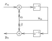
(i) State the equations that define the elements of the output sequence  $\{y_n\}$ and the intermediate sequence  $\{u_n\}$  in terms of other values from  $\{x_n\}$ ,  $\{y_n\}$  or  $\{u_n\}$ . [4 marks]
