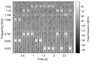
The manual of the recorder does not explain what the "scramble" switch does. Using a spectrogram (above), you spot at the start of the recording a sequence of 14 tone pairs.
