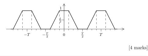
Answer: We can obtain q(t), which has a high/low transition time of T/4, by convolving p(t) from part (b) with a rectangular window of width T/4:
