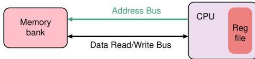
Single-core, basic computer model (no hardware concurrency).
