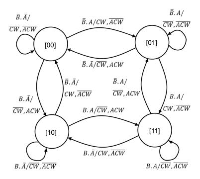
FF labels:  $[Q_B Q_A]$  Transition labels: Inputs/Outputs
