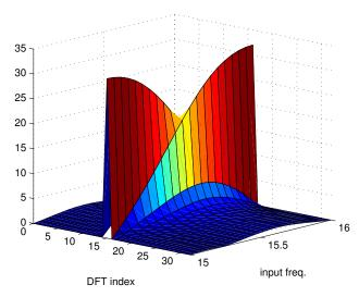
The *leakage* of energy to other frequency bins not only blurs the estimated spectrum. The peak amplitude also changes significantly as the frequency of a tone changes from that associated with one output bin to the next, a phenomenon known as *scalloping*. In the above graphic, an input sine wave gradually changes from the frequency of bin 15 to that of bin 16 (only positive frequencies shown).
