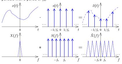
A signal x(t) that is sampled with frequency  $f_s$  has a spectrum that is periodic with a period of  $f_s$ .
