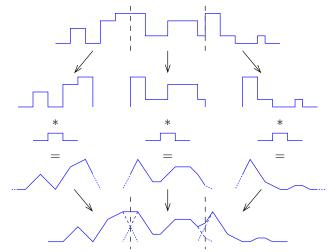
The regions originally added as zero padding are, after convolution, aligned to overlap with the unpadded ends of their respective neighbour blocks. The overlapping parts of the blocks are then added together.
