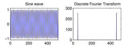
Sine wave multiplied with window function Discrete Fourier Transform
