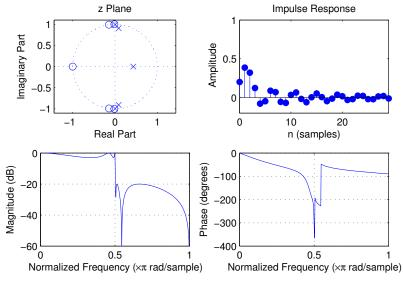
order: 5, cutoff frequency: 0.5  $\times$   $f_{\rm s}/2,$  pass-band ripple: -3 dB, stop-band ripple: -20 dB
