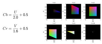
Modern image compression techniques operate on Y, Cr, Cb channels separately, using half the resolution of Y for storing Cr, Cb.
