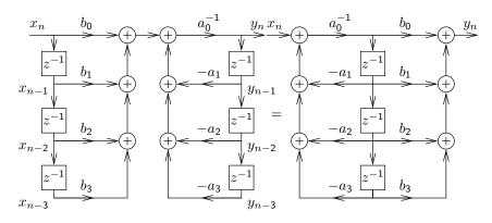
The block diagram representation of the constant-coefficient difference equation on slide 25 is called the *direct form I implementation*.
