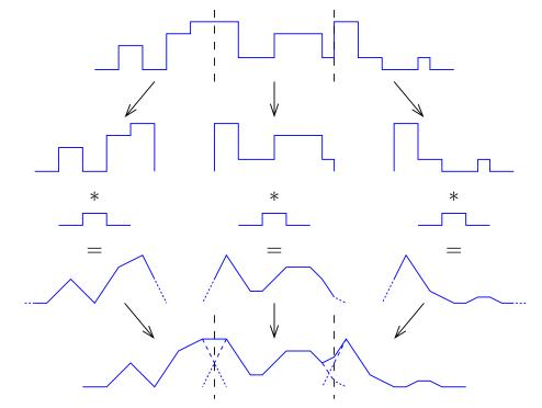
The regions originally added as zero padding are, after convolution, aligned to overlap with the unpadded ends of their respective neighbour blocks. The overlapping parts of the blocks are then added together.
