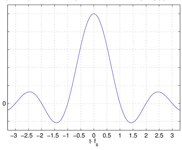
Impulse response of ideal low-pass filter with cut-off frequency  $f_s/2$ :
