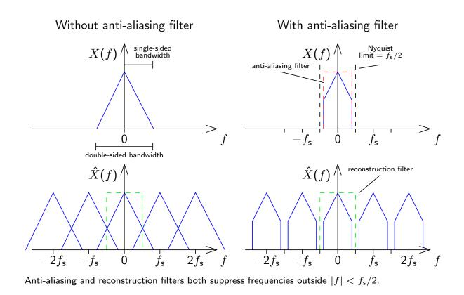
Reconstruction of a continuous band-limited waveform
