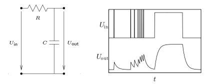
Any passive network (resistors, capacitors, inductors) convolves its input voltage  $U_{in}$  with an *impulse response function* h, leading to  $U_{out} = U_{in} * h$ , that is
