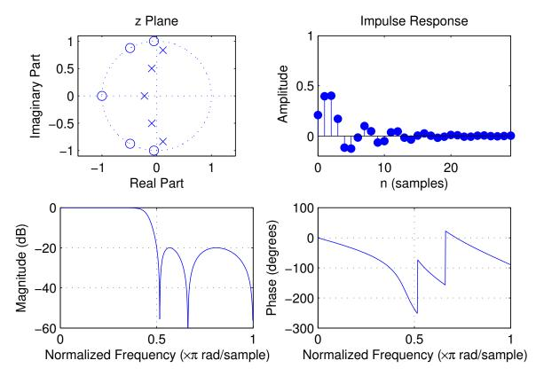
order: 5, cutoff frequency: 0.5 imes  $f_{\rm s}/2$ , stop-band ripple: -20 dB
