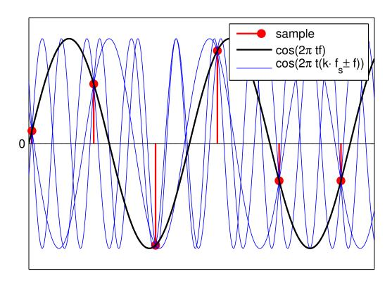
Sampled at frequency  $f_s$ , the function  $\cos(2\pi t f)$  cannot be distinguished from  $\cos[2\pi t(kf_s \pm f)]$  for any  $k \in \mathbb{Z}$ .
