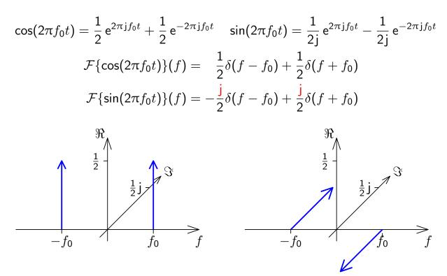
As any  $x(t) \in \mathbb{R}$  can be decomposed into sine and cosine functions, the spectrum of any real-valued signal will show the symmetry  $X(-f) = [X(f)]^*$ , where \* denotes the complex conjugate (i.e., negated imaginary part).
