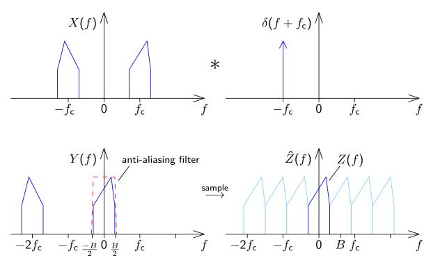
Shifting the center frequency  $f_c$  of the interval of interest to 0 Hz (DC) makes the spectrum asymmetric. This leads to a complex-valued time-domain representation  $(\exists f: Z(f) \neq [Z(-f)]^* \Longrightarrow \exists t: z(t) \in \mathbb{C} \setminus \mathbb{R}).$
