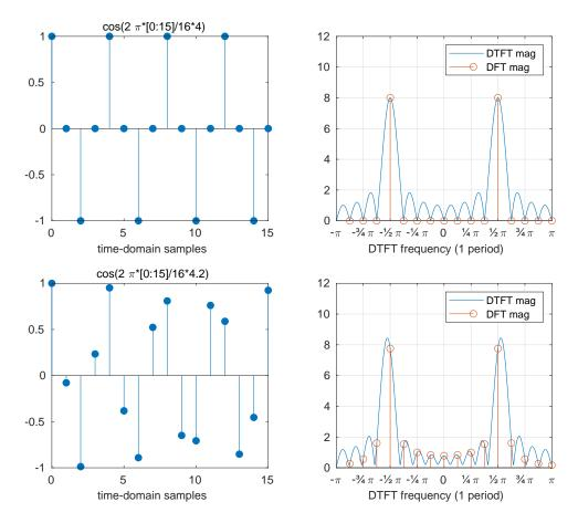
We introduced the DFT as a special case of the continuous Fourier transform, where the input is sampled *and periodic*.
