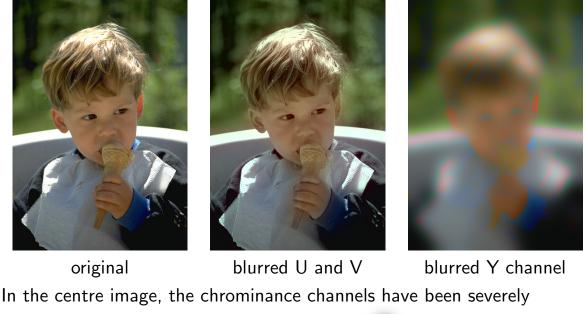
low-pass filtered (Gaussian impulse response ). But the human eye perceives this distortion as far less severe than if the exact same filtering is applied to the luminance channel (right image).
