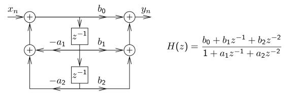
Filter sections  $H_1, H_2, \ldots, H_l$  are then applied sequentially to the input sequence, resulting in a filter
