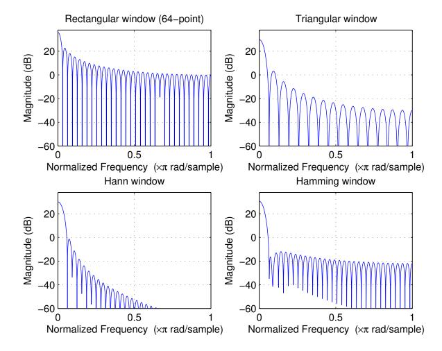
Numerous alternatives to the rectangular window have been proposed that reduce leakage and scalloping in spectral estimation. These are vectors multiplied element-wise with the input vector before applying the DFT to it. They all force the signal amplitude smoothly down to zero at the edge of the window, thereby avoiding the introduction of sharp jumps in the signal when it is extended periodically by the DFT.
