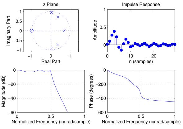
order: 5, cutoff frequency: 0.5 imes  $f_{\rm s}/2$ , pass-band ripple: -3 dB
