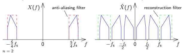
In this case, the aliasing copies of the positive and the negative frequencies will interleave instead of overlap, and can therefore be removed again later by a reconstruction filter.
