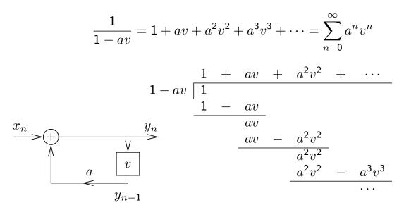
Rational functions (quotients of two polynomials) can provide a convenient closed-form representations for infinitely-long exponential sequences, in particular the impulse responses of IIR filters.
