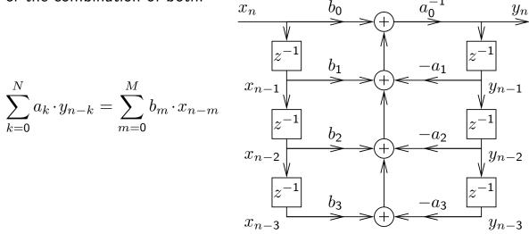
Implementations: DSP.jl's filt(b, a, x), MATLAB's filter, scipy.signal.lfilter.
