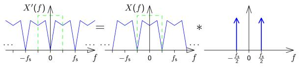
This can be accomplished by multiplying the sampled sequence  $x_i$  with  $y_i = \cos \pi f_s t = \cos \pi i = e^{j\pi i}$ , which is nothing but multiplication with the sequence
