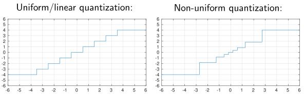
Quantization is the mapping from a continuous or large set of values (e.g., analog voltage, floating-point number) to a smaller set of (typically  $2^8$ ,  $2^{12}$  or  $2^{16}$ ) values.
