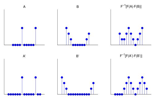
Both sequences are padded with zero values to a length of at least m + n - 1. This ensures that the start and end of the resulting sequence do not overlap.
