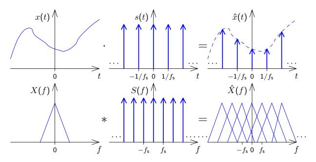
Sampling a signal in the time domain corresponds in the frequency domain to convolving its spectrum with a Dirac comb. The resulting copies of the original signal spectrum in the spectrum of the sampled signal are called "images".
