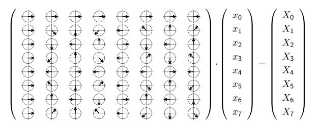
The *n*-point DFT of a signal  $\{x_i\}$  sampled at frequency  $f_s$  contains in the elements  $X_0$  to  $X_{n/2}$  of the resulting frequency-domain vector the frequency components 0,  $f_s/n$ ,  $2f_s/n$ ,  $3f_s/n$ , ...,  $f_s/2$ , and contains in  $X_{n-1}$  downto  $X_{n/2}$  the corresponding negative frequencies. Note that for a real-valued input vector, both  $X_0$  and  $X_{n/2}$  will be real, too. Why is there no phase information recovered at  $f_s/2$ ?
