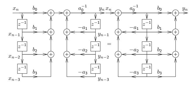
The block diagram representation of the constant-coefficient difference equation on slide 25 is called the *direct form I implementation*.
