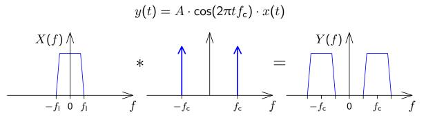
The spectrum of the baseband signal in the interval  $-f_{\rm I} < f < f_{\rm I}$  is shifted by the modulation to the intervals  $\pm f_{\rm c} - f_{\rm I} < f < \pm f_{\rm c} + f_{\rm I}$ . How can such a signal be demodulated?
