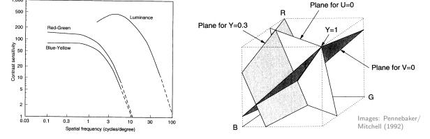
The human eye processes colour and luminosity at different resolutions. To exploit this phenomenon, many image transmission systems use a colour space with a "luminance" coordinate
