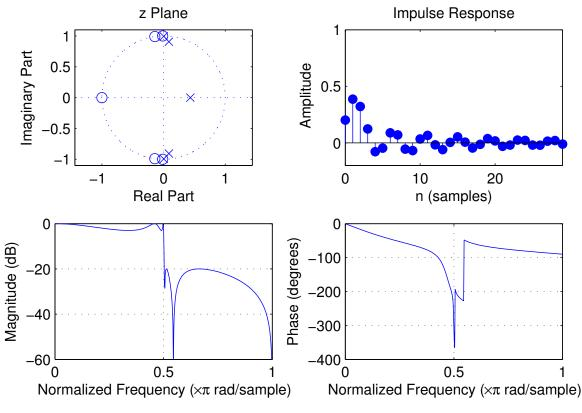
order: 5, cutoff frequency: 0.5 imes  $f_{s}/2$ , pass-band ripple: -3 dB, stop-band ripple: -20 dB
