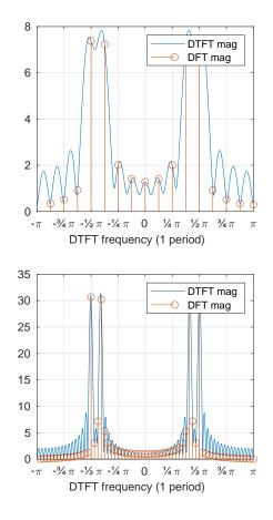
Applying the discrete Fourier transform (DFT) to an *n*-element long real-valued sequence samples the DTFT of that sequence at n/2 + 1 discrete frequencies.
