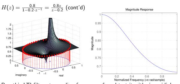
Run this LTI filter at sampling frequency  $f_s$  and test it with sinusoidial input (frequency f, amplitude 1):  $x_n = \cos(2\pi f n/f_s)$ Output:  $y_n = A(f) \cdot \cos(2\pi f n/f_s + \theta(f))$ What are the gain A(f) and phase delay  $\theta(f)$  at frequency f? Answer:  $A(f) = |H(e^{j2\pi f/f_s})|$  $\theta(f) = \angle H(e^{j2\pi f/f_s}) = \tan^{-1} \frac{\Im\{H(e^{j2\pi f/f_s})\}}{\Re\{H(e^{j2\pi f/f_s})\}} + k\pi$  angle  $\tan^2$  $\operatorname{unwrap}$
