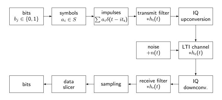
IQ up/down conversion: only required for pass-band channels (e.g., radio)
