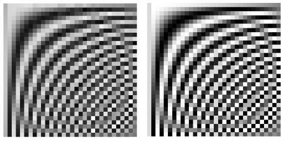
**Breakthrough:** Ahmed/Natarajan/Rao discovered the DCT as an excellent approximation of the KLT for typical photographic images, but far more efficient to calculate.
