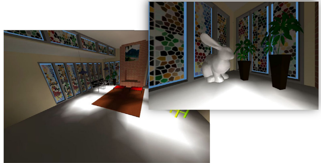
Step 4: Render the scene using interpolated values from the irradiance probes to look up indirect illumination
