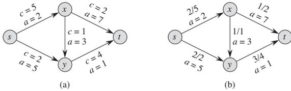
**Figure 29.3** (a) An example of a minimum-cost-flow problem. We denote the capacities by  $c$  and the costs by  $a$ . Vertex  $s$  is the source and vertex  $t$  is the sink, and we wish to send 4 units of flow from  $s$  to  $t$ . (b) A solution to the minimum-cost flow problem in which 4 units of flow are sent from  $s$  to  $t$ . For each edge, the flow and capacity are written as flow/capacity.
