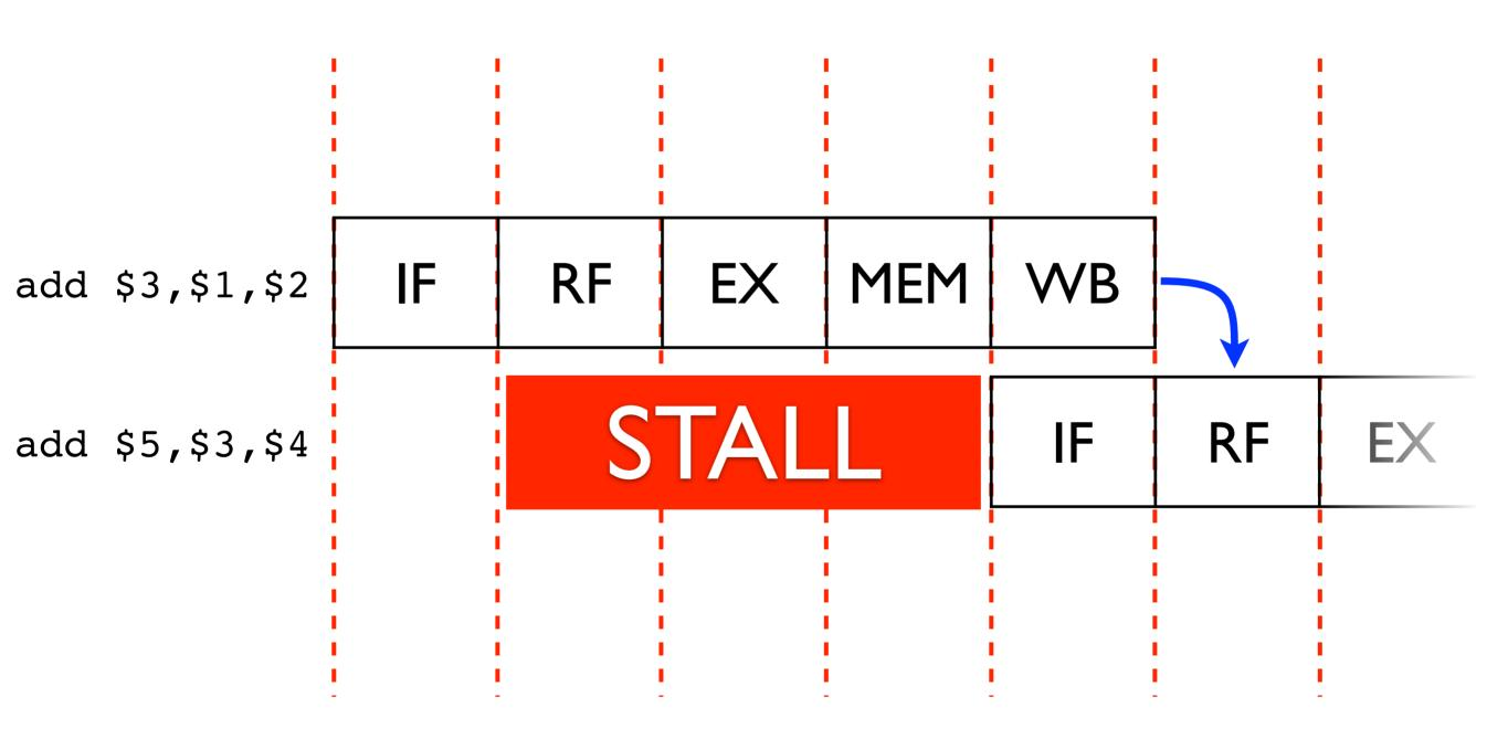
The severity of this effect can be reduced by using bypassing: extra paths are added between functional units, allowing data to be used before it has been written back into registers.
