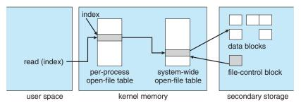
Using per-process open-file table, index (file handle or file descriptor) resolves to system-wide open-file table containing file-control block which resolves to actual data blocks on disk
