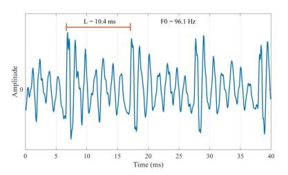
Segment of a speech signal, with the period length *L*, and fundamental frequency FO=1/L.
