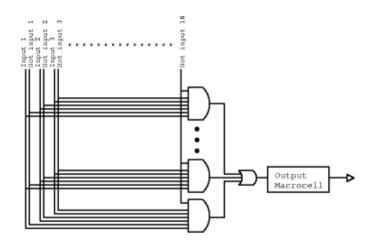
The output from the each OR gate is connect to an output pin through an output macrocell. This can be programmed to latch (using a D-type FF) the output or feed the output signal back into AND array. For a more detailed description of this PAL, read the datasheet.
