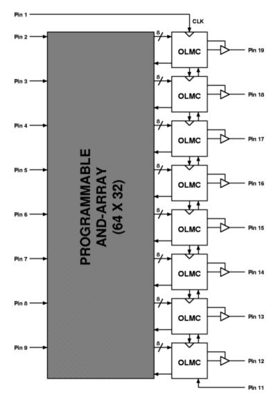
The equations for each output (called P19 to P12, in that order) can consist of inputs, operators and brackets. The input must be referred to by the "P" followed by a number. Operators are &, |, and ! for AND, OR, and NOT respectively.
