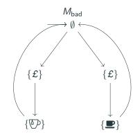
A G ( $\mathcal{E} \to E \times \mathbb{P}$ ): "For all paths, at every state (along the path) in which money has been paid, there exists a path from this state in which, in the next state, the machine has produced coffee."
