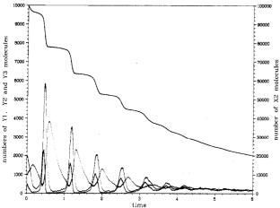
Figure 27. Showing what would have happened in the run of Figure 24 if the system had been closed to species  $X_2$ . All trajectories are plotted at 100 rpd. The heavy decaying curve is  $X_2$ , and the low-peaking, middle-peaking, and high-peaking curves are  $Y_1$ ,  $Y_2$ , and  $Y_3$ , respectively
