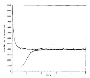
**Figure 7.** A 40 rpd plot of two stochastic simulation runs for reactions 29, with  $c_1X = 5$  and  $c_2 = 0.00125$ , corresponding to the deterministic steady state Y = 4000; one run starts at Y = 40, and the other run starts at Y = 12000.
