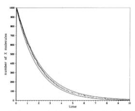
**Figure 3.** The one-standard deviation envelope (dashed) and two-standard deviation envelope (solid) as calculated from the master equation, superimposed on the results of one stochastic simulation run (dots), of the simple isomerization reaction (22) with c=0.5 and  $X_0=1000$ . The simulation run is plotted at 1 rpd (reactions per dot).
