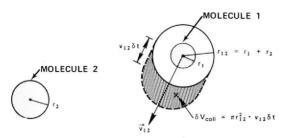
**Figure 1.** The "collision volume"  $\delta V_{\rm coll}$  which molecule 1 will sweep out relative to molecule 2 in the next small time interval  $\delta t$ .
