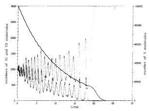
**Figure 10.** Combined 100 rpd plots of X (dark curve),  $Y_1$  (upper oscillating curve), and  $Y_2$  (lower oscillating curve) vs. t for a stochastic simulation run of the *closed* Lotka reactions, with  $c_1 = 0.0001$ ,  $c_2 = 0.01$ , and  $c_3 = 10$ .
