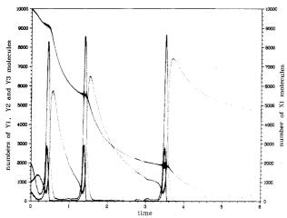
Figure 26. Showing what would have happened in the run of Figure 24 if the system had been closed to species  $X_1$ . All trajectories are plotted at 100 rpd. The decaying curve is  $X_1$ , and the low-peaking, middle-peaking, and high-peaking curves are  $Y_1$ ,  $Y_2$ , and  $Y_3$  respectively.
