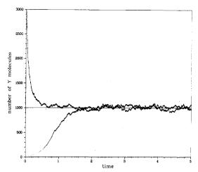
**Figure 6.** A 10 rpd plot of two stochastic simulation runs for reactions 29, with  $c_1X = 5$  and  $c_2 = 0.005$ , corresponding to the deterministic steady state Y = 1000; one run starts at Y = 10, and the other run starts at Y = 3000.
