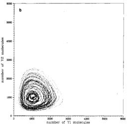
**Figure 12.** Results of a 1.5  $\times$  10<sup>6</sup> reaction stochastic simulation run of the Lotka reactions *including* reaction 38d, with  $c_1 = 0.0002$ ,  $c_2 = 0.01$ ,  $c_3 = c_4 = 10$ , and  $X = 10^5$  (constant), corresponding to the deterministic steady-state  $Y_1 = Y_2 = 1000$ . (a) A 200 rpd plot of  $Y_1$  vs. t for  $0 \le t \le 30$ . (b) A 200 rpd plot of  $Y_2$  vs.  $Y_1$  for  $0 \le t \le 30$ . of  $Y_2$  through natural causes.
