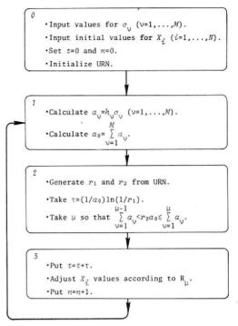
Figure 2. Schematic of the stochastic simulation algorithm.
