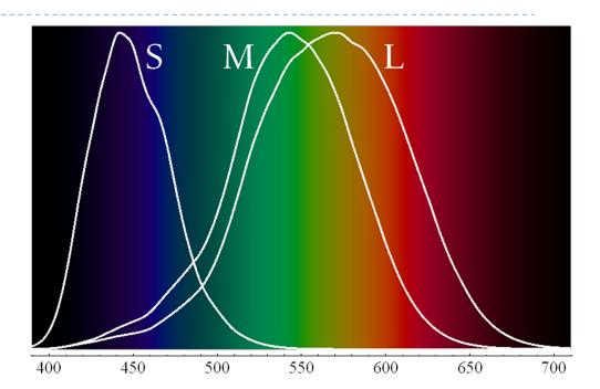
Sensitivity curves – probability that a photon of that wavelengths will be absorbed by a photoreceptor. S,M and L curves are normalized in this plot.
