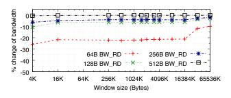
Figure 8: Difference between local and remote DMA Reads of different sizes with warm cache (NFP6000-BDW).
