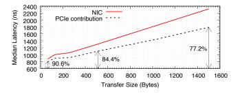
Figure 2: Measurement of NIC PCIe latency.
