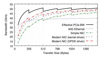
Figure 1: Modeled bidirectional bandwidth of a PCIe Gen 3 x8 link, the achievable throughout of a simplistic NIC and a modern NIC with a typical kernel driver and a DPDK driver.
