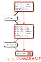
On *this* path through the flowgraph, x+y is only computed once, so x+y is *syntactically* unavailable at the last instruction.
