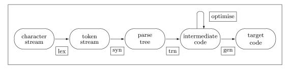
This course only considers the optimiser, which in principle is both source-language and target-architecture independent, but certain gross target features may be exploited (e.g. number of user allocatable registers for a register allocation phase).
