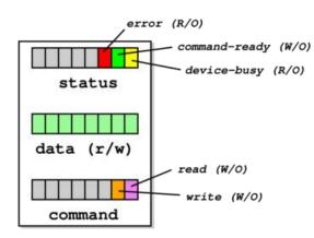
Consider a simple device with three registers: status, data and command. Host can read and write these via bus. Then polled mode operation works as follows:
