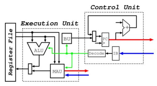
result. If **Branch Unit** (BU), test condition and (maybe) add value to PC. If **Memory Access Unit** (MAU), generate address ("addressing mode") and use bus to read/write value
