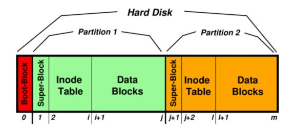
A disk consists of a boot block followed by one or more partitions. Very old disks would have just a single partition. Nowadays have a **boot block** containing a partition table allowing OS to determine where the filesystems are
