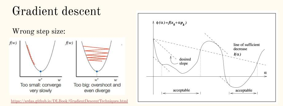
Line search converges to the minimizer when the iterates follow the Wolfe conditions on sufficient decrease and curvature (Zoutendijk's theorem)
