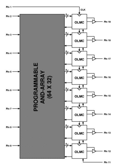
The equations for each output (called P19 to P12, in that order) can consist of inputs, operators and brackets. The input must be referred to by the "P" followed by a number. Operators are &, |, ^ and ! for AND, OR, XOR and NOT respectively
