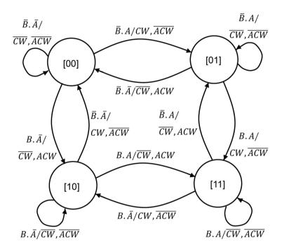
FF labels:  $[Q_B Q_A]$  Transition labels: Inputs/Outputs
