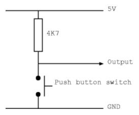
Note: The 4K7 resistor is often known as a 'pull-up' resistor since the Output is pulled-up to 5V when the push button switch is open (not pressed).
