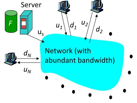
$$d_{P2P} = \max \{ F/u_s, F/min(d_i), NF/(u_s + \Sigma u_i) \}$$
