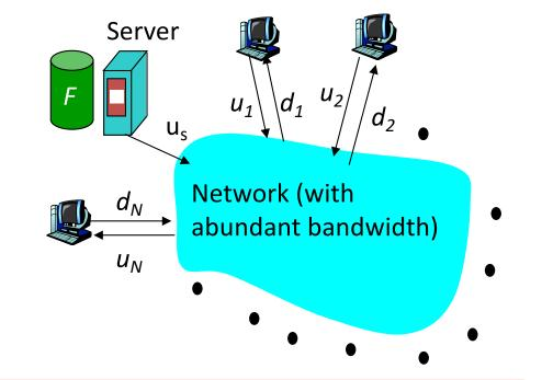
Time to distribute F to N clients using = d<sub>cs</sub> = max { NF/u<sub>s</sub>, F/min(d<sub>i</sub>) } client/server approach i
