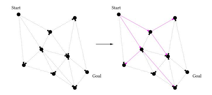
The graph becomes *separated*: any path from the start to an unexplored node *has to pass through a fringe node*.
