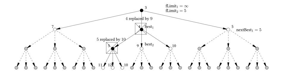
Now  $f(\text{best}_2) > \text{fLimit}_2$  so the function call returns (NONE, 9) into (result<sub>2</sub>, f') and  $f(\text{best}_1) = 9$ .
