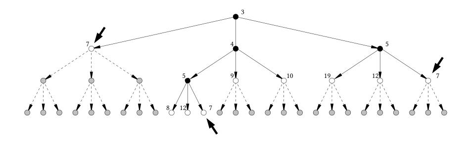
The new limit is 7, so at the next iteration the three arrowed nodes will be explored.
