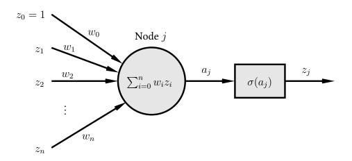
Weights  $w_i$  connect nodes together, and  $a_j$  is the weighted sum or activation for node j.  $\sigma$  is the activation function and the output is  $z_j = \sigma(a_j)$ .
