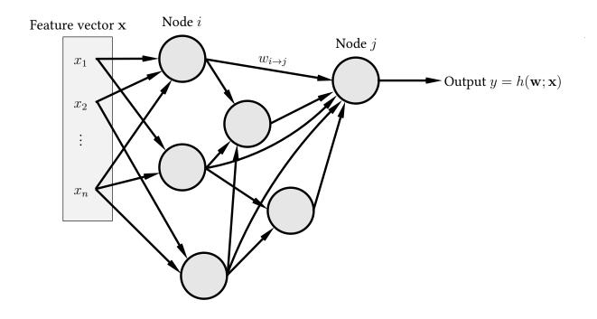
*Each node* is a perceptron. *No specific layering* is assumed.  $w_{i\rightarrow j}$  connects node i to node j.  $w_0$  for node j is denoted  $w_{0\rightarrow j}$ .
