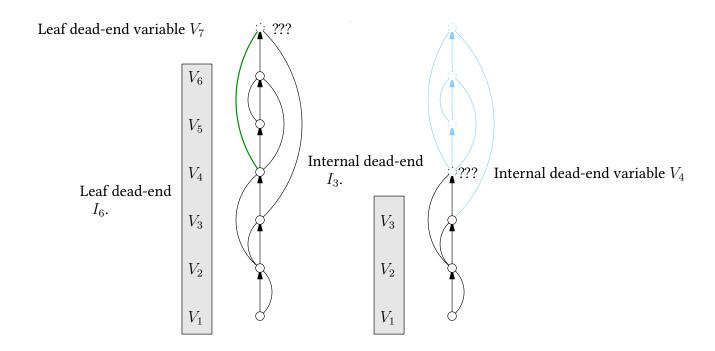
If  $V_i$  was backtracked to from a later leaf dead-end and there are no more values to try for  $V_i$  then we refer to it as an *internal dead-end variable* and call  $I_{i-1}$  an *internal dead-end*.
