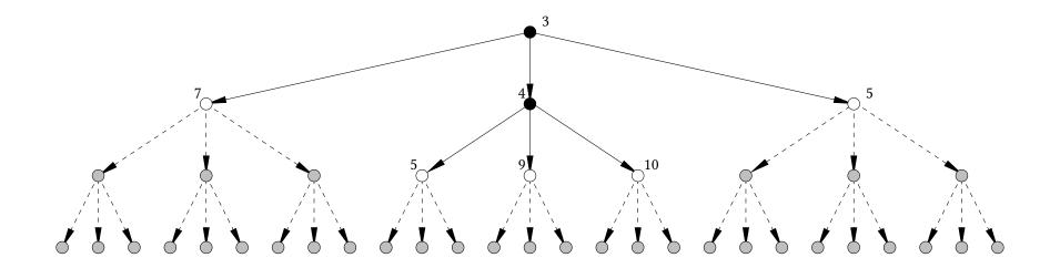
Anything with f cost at most equal to the current limit gets explored, and the algorithm keeps track of the *smallest* f cost that is greater than its current limit. The new limit is 5.
