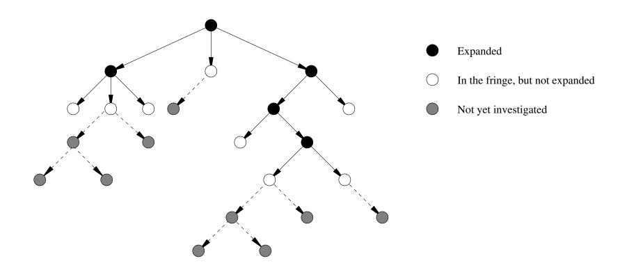
At each iteration, one node from the fringe is expanded. In general, if the *branching factor* is b then the *layer* at *depth* d can have  $b^d$  states.
