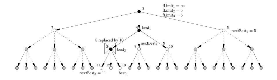
Now  $f(\text{best}_3) > \text{fLimit}_3$  so the function call returns (NONE, 10) into (result<sub>3</sub>, f') and  $f(\text{best}_2) = 10$ .
