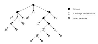
At each iteration, one node from the fringe is expanded. In general, if the *branching factor* is b then the *layer* at *depth* d can have  $b^d$  states.
