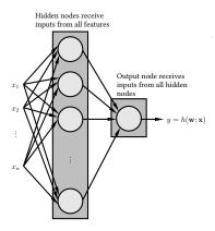
For the output:  $\sigma(a)=a.$  For the hidden nodes  $\sigma(a)=\frac{1}{1+\exp(-a)}$
