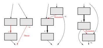
A planner can try to fix a threat by introducing an ordering constraint.
