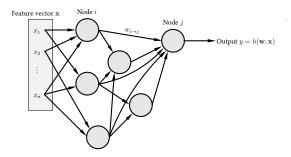
Each node is a perceptron. No specific layering is assumed.  $w_{i\rightarrow j}$  connects node i to node j.  $w_0$  for node j is denoted  $w_{0\rightarrow j}$ .
