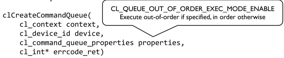
Provides means to both synchronize kernels and execute them in parallel
