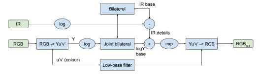
The RGB image is decomposed into luminance (Y) and chrominance (u'v') channels. Because HVS is not sensitive to the loss of high frequencies in chrominance (HVS lecture), chrominance channels can be low-pass filtered to reduce noise. The luminance and IR channels are
