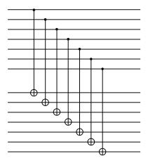
This is fault tolerant, as each of the component CNOT gates acts on exactly one qubit in the first block and one qubit in the second block. Therefore a single error will propagate to (at most) one qubit in each block, as per the definition of fault tolerant quantum gates.
