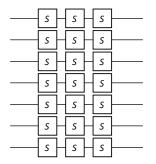
Again, this is fault tolerant as each component physical S gate acts on a single qubit.
