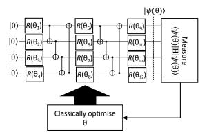
Here we can see that the quantum circuit takes the form of a parameterised quantum circuit (PQC), or variational quantum circuit. There are many forms of PQC, in this sketch we show one where entangling CNOT gates are interspersed with parameterised rotation gates. PQCs are sometimes described as quantum analogues of neural networks, and are also used in quantum machine learning.
