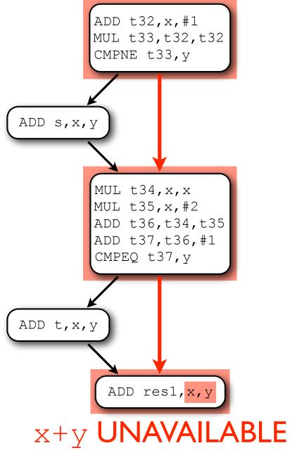
On this path through the flowgraph, x+y is only computed once, so x+y is syntactically unavailable at the last instruction.
