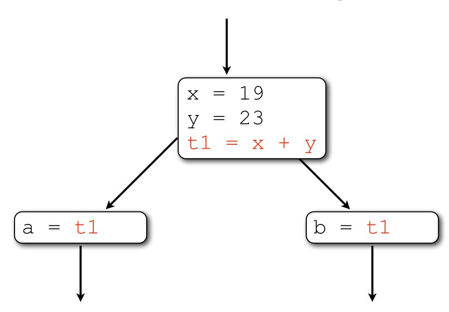
Hoisting may have a different effect on execution time depending on the exact nature of the code. The resulting program may be slower, faster, or just the same speed as before.
