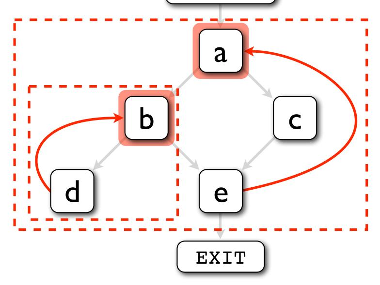
Once each loop has been identified, we can examine its structure to determine what kind of loop it is, and hence how best to represent it in source code.
