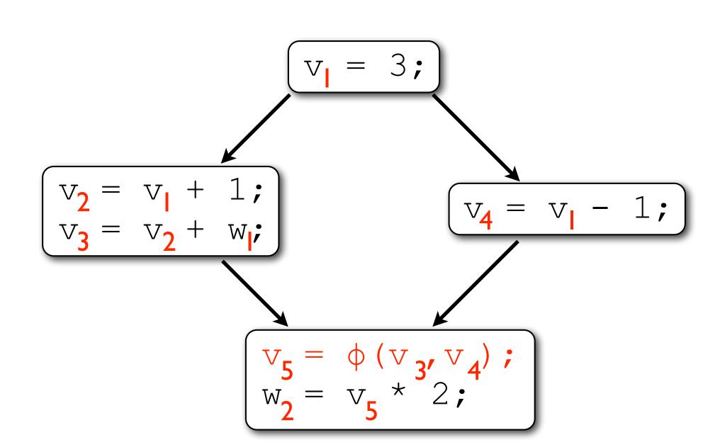
The φ-functions in SSA keep track of which variables are merged at control-flow join points.
