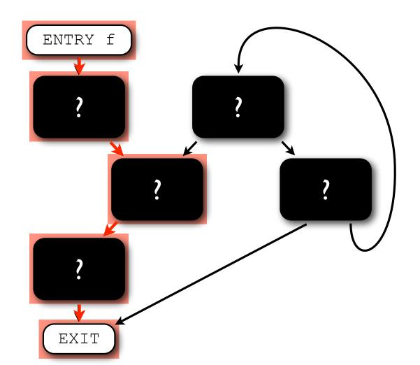
For example, straightening is an optimisation which can eliminate jumps between basic blocks by coalescing them:
