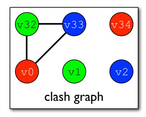
This final technique of synthesising edges on the clash graph in order to avoid corrupted registers is helpful for dealing with the procedure calling standard of the target architecture.
