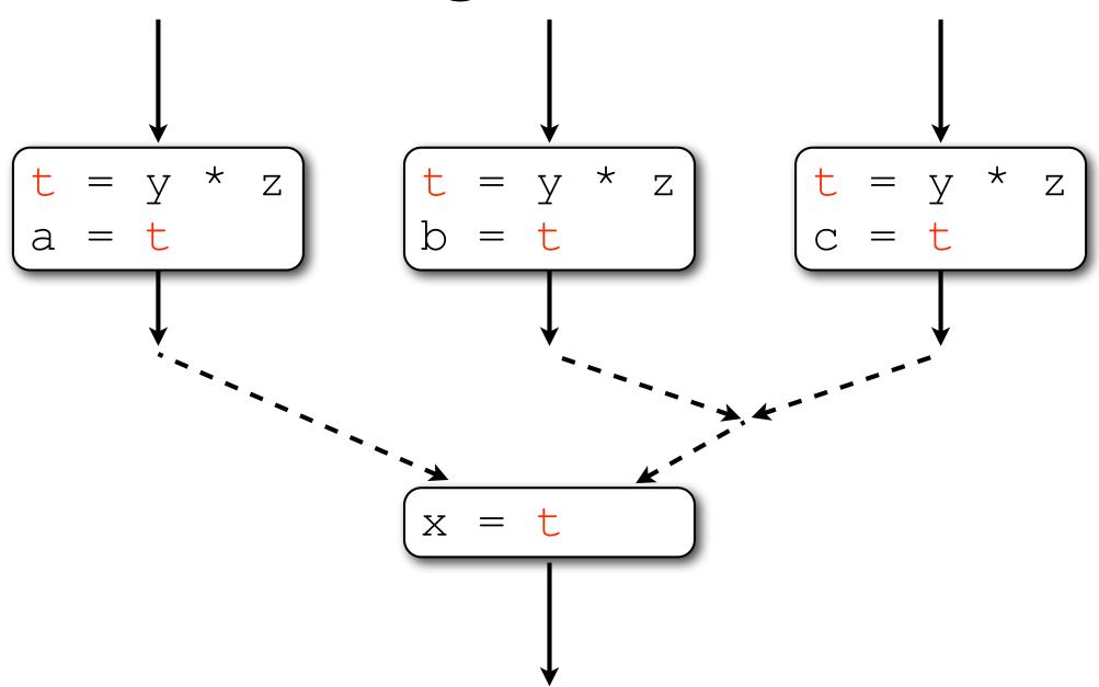
Our transformed program performs (statically) fewer arithmetic operations: y\*z is now computed in three places rather than four.
