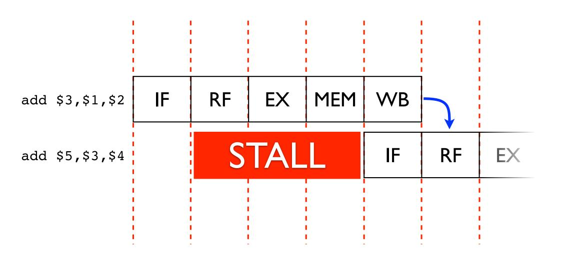
The severity of this effect can be reduced by using bypassing: extra paths are added between functional units, allowing data to be used before it has been written back into registers.
