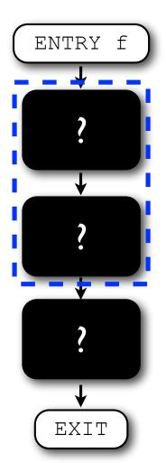
For example, straightening is an optimisation which can eliminate jumps between basic blocks by coalescing them:
