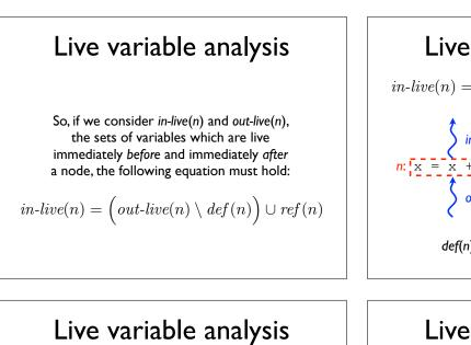
So we know how to calculate *in-live*(*n*) from the values of *def*(*n*), *ref*(*n*) and *out-live*(*n*). But how do we calculate *out-live*(*n*)?
