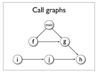
Call graphs Again, the precision of the graph is compromised in the presence of indirect calls. ENTRY f ENTRY main MOV t33,<mark>#</mark>&f EXIT ENTRY g MOV t34,<mark>#&g</mark> MOV t35,<mark>#</mark>&h EXIT CALLI t32 ENTRY h 2 EXIT EXIT
