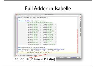
The logical formula above is a direct translation of the diagram on the previous slide. Needless to say, the translation from diagram to formula should ideally be automatic, and better still, driven by the same tools that fabricate the actual chip.
