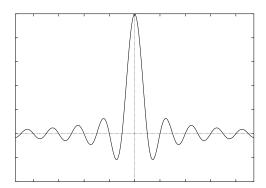
(e) Explain why smoothing a signal, by low-pass filtering it before sampling it, can prevent aliasing. Explain aliasing by a picture in the Fourier domain, and also show in the picture how smoothing solves the problem. What would be the most effective low-pass filter to use for this purpose? Draw its spectral sensitivity.
