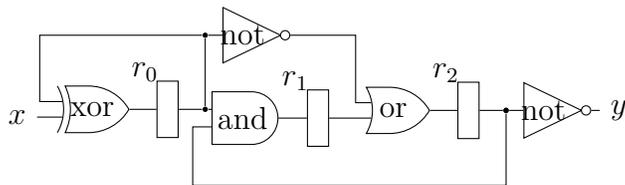
Assuming registers  $r_0$  and  $r_2$  are initially both set to 1, and  $r_1$  is initially set to 0:
