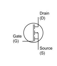
The current flow from S to D ( $I_{DS}$ ) is controlled by the voltage applied between G and S ( $V_{GS}$ ), i.e., G has to be -ve wrt S for current  $I_{DS}$  to flow (transistor **On**)
