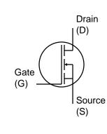
The current flow from D to S ( $I_{DS}$ ) is controlled by the voltage applied between G and S ( $V_{GS}$ ), i.e., G has to be +ve wrt S for current  $I_{DS}$  to flow (transistor **On**)
