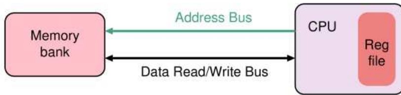
Single-core, basic computer model (no hardware concurrency).
