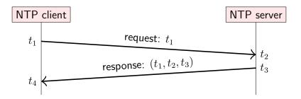
Round-trip network delay:  $\delta = (t_4 - t_1) - (t_3 - t_2)$
