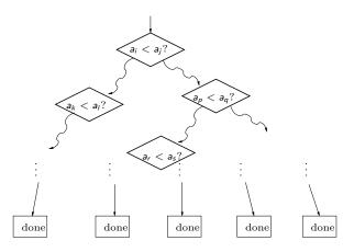
To work for all permutations of the input list, the tree must have at least n! leaves and therefore height at least  $\log_2(n!) = \theta(n \log n)$ .
