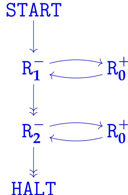
**Claim:** starting from initial configuration  $(0, 0, x, y)$ , this machine's computation halts with configuration  $(4, x + y, 0, 0)$ .
