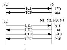
Figure 6. Message flow for a successful user search when SC v1.4 is behind a port-restricted NAT. 'B' stands for bytes and 'N' stands for node. UDP packets were sent to N1, N2, N3, and N4 during login process and responses were received from them. Message size corresponds to payload size of TCP or UDP packets. Not all messages are shown.
