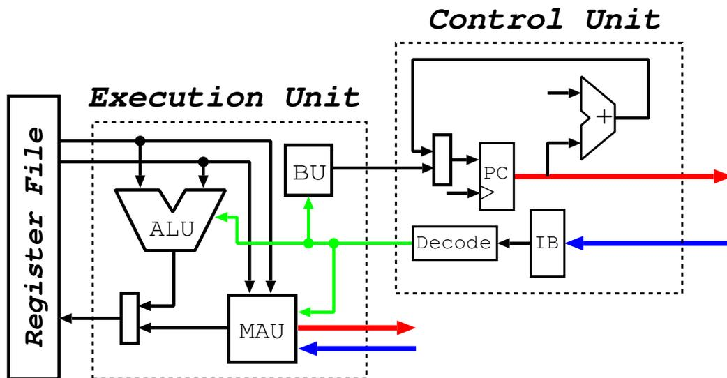
1. CU fetches & decodes instruction and generates (a) control signals and (b) operand information.
