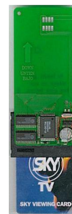
Conductive silver ink attack on BSKyB P10 card (top), with card CPU replaced by external DS5002FP (right)
