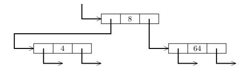
The tree is built up one node at a time. A new node is put on the tree in such a way that the tree is ordered. Thus 4 < 8 < 64. If the next new node is to incorporate 32, it will hang from the left of the 64 node.
