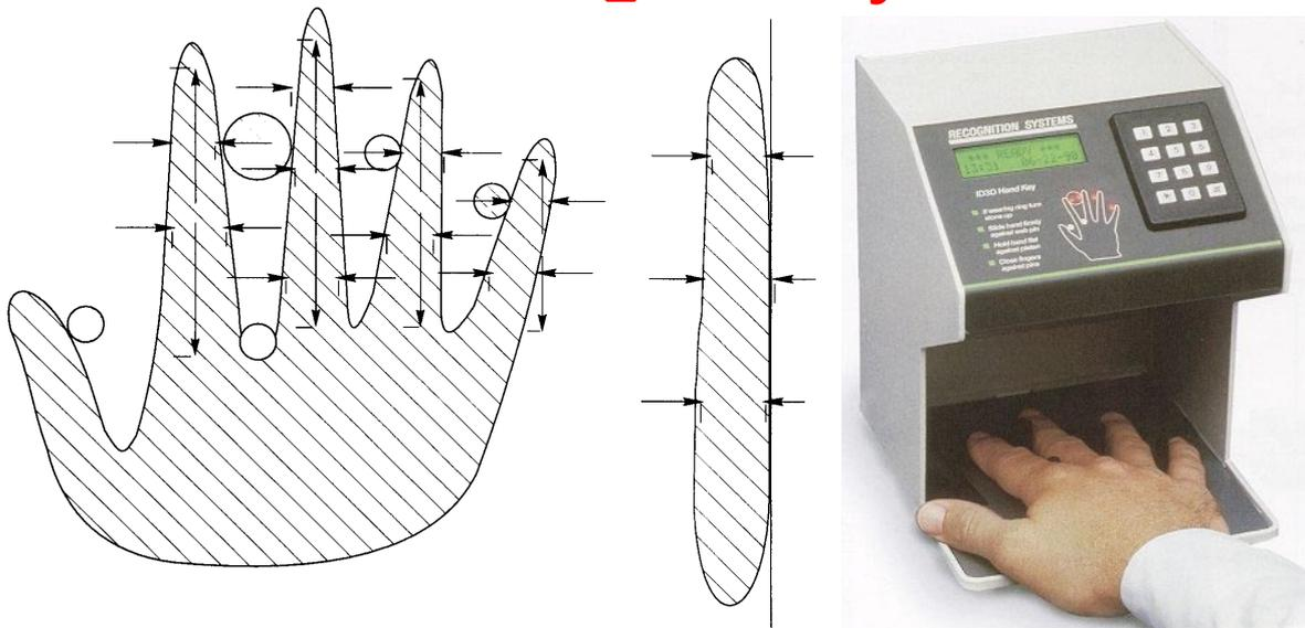
Biometric characteristic used are several dozen length and thickness measurements of the fingers. Digital camera captures two hand silhouettes. Hand needs to be aligned to posts, which may require some practice and good hand mobility.
