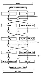
The round function f expands the 32-bit input to 48-bit, XORs this with a 48-bit subkey, and applies eight carefully designed 6-bit to 4-bit substitution tables ("s-boxes"). The expansion function E makes sure that each sbox shares one input bit with its left and one with its right neighbour.
