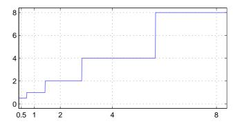
Example for non-uniform quantization: digital telephone network
