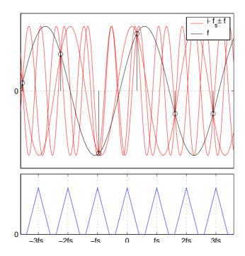
A wave  $\cos(2\pi t f)$  sampled with frequency  $f_s$  cannot be distinguished from  $\cos(2\pi t (i f_s \pm f))$  for any  $i \in \mathbb{Z}$ , therefore ensure  $|f| < f_s/2$ .
