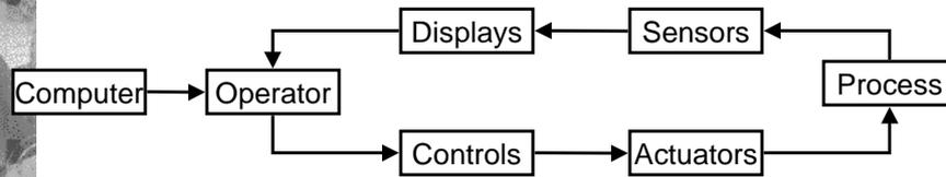
(a) Computer provides information and advice to controller, perhaps by reading sensors directly
