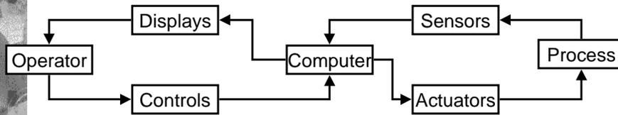
(c) Computer interprets and displays data for operator and issues commands; operator makes varying levels of decisions)
