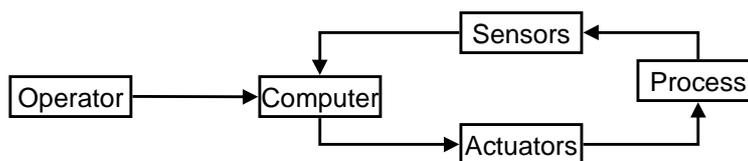
(d) Computer assumes complete control of process with operator providing advice or high-level direction
